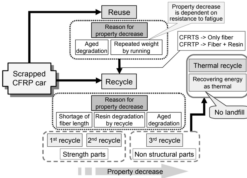
Fig.2 Reuse and recycle flow of scrapped CFRP cars in the future
