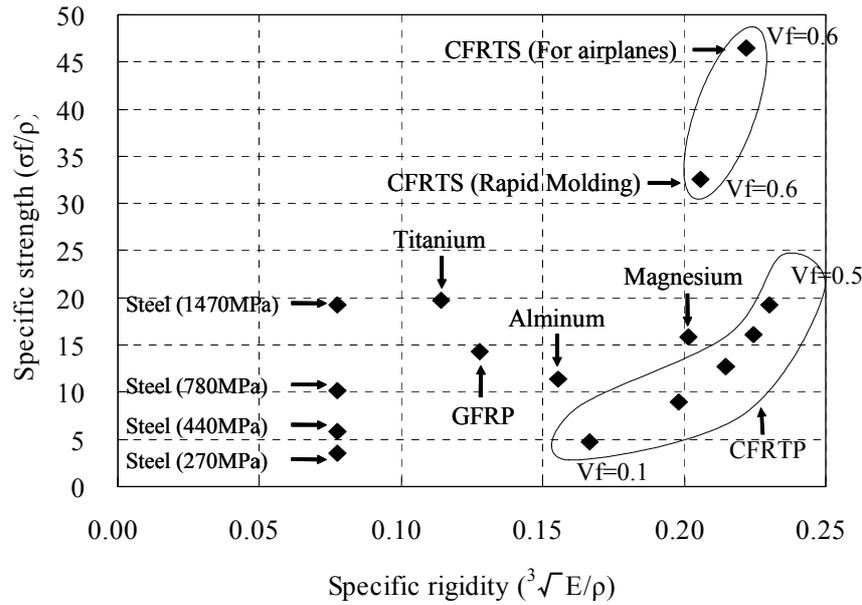
Fig.1 Specific rigidity and specific strength of various materials
