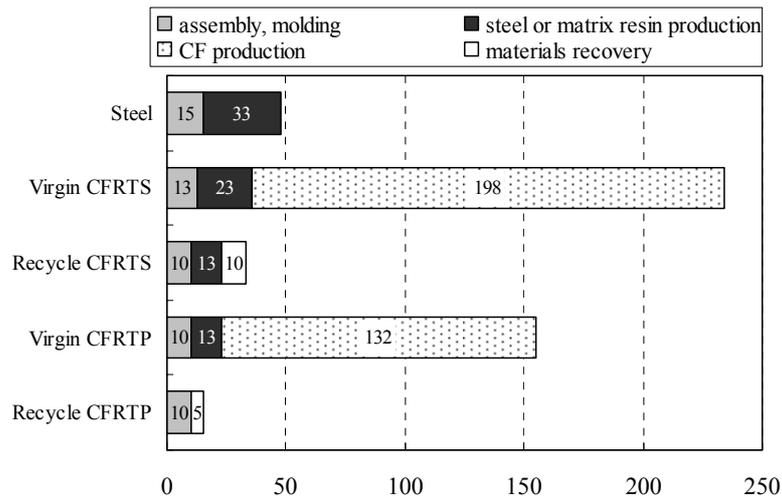
Fig.3 Energy intensity (MJ/kg) of virgin and recycled materials
