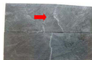
Fig. 3 Breaking section of recycled CMT
