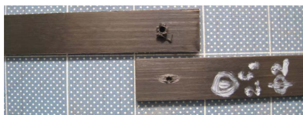
(a) Oscillation time of 2.5 sec with horn diameter of 2 mm.
