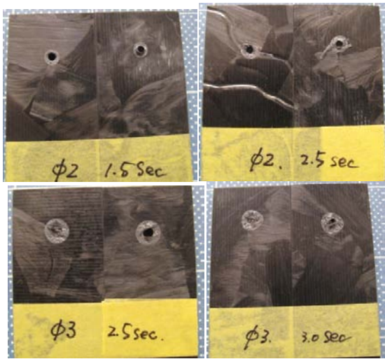
Fig. 11 Joint part of single lap specimens by spot welding (Random)
