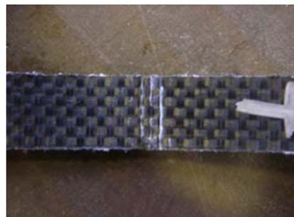
Fig. 15 Failure of CF/PP at strain of 3.7% (compressive side).
