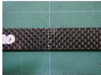
Fig. 14 Failure of CF/EP at ult. load (compressive side).
