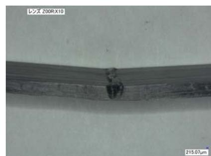
Fig. 7 Failure of CF/PP at strain of 3.0%.
