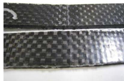
Fig. 16 Thermally repaired specimen and damaged specimen.
