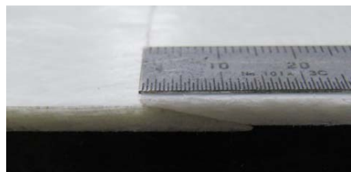
Fig. 1 Tapered jointing section
