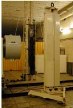
FIG. 6. (Color) Collimation system forming a 4 mm fan-shaped beam.
