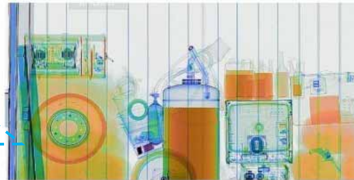
FIG. 13. (Color) Colorized image of a shipping container with color assignment according to Table II. Colorization is fulfilled after the segmentation procedure.
