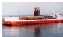
“Sagar-Shakthi” 1MW Closed Cycle OTEC power plant 佐賀大学とインドNITOT
