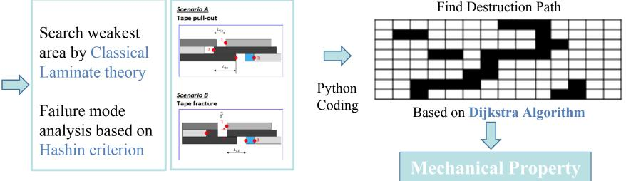
Aim to provide a reliable means to predict CTT property according the input parameters.
