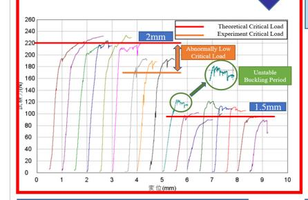
Output: Predict Buckling Failure
