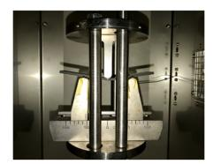
Three-point bending test DSC Test SEM
