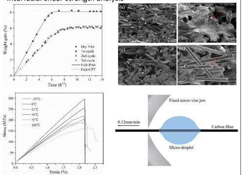
The performance of CFRTP in moisture, sea water, hydrothermal environment, thermo-oxidation has been confirmed. The application of this material in marine field and fire-fighting field is expected.
