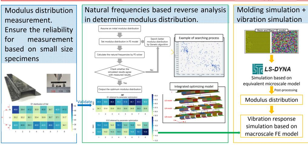
Accurate vibration response simulation → Contribute to the vibration control and fatigue lifespan design for automobile development when CTT is applied
