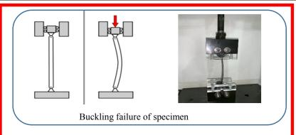
Problem: the anisotropic property of the CTT materials makes it hard for designers to predict the buckling failure of a certain mechanism.
